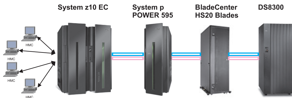
Figure 20. The Insurance Company hardware configuration before zEnterprise
